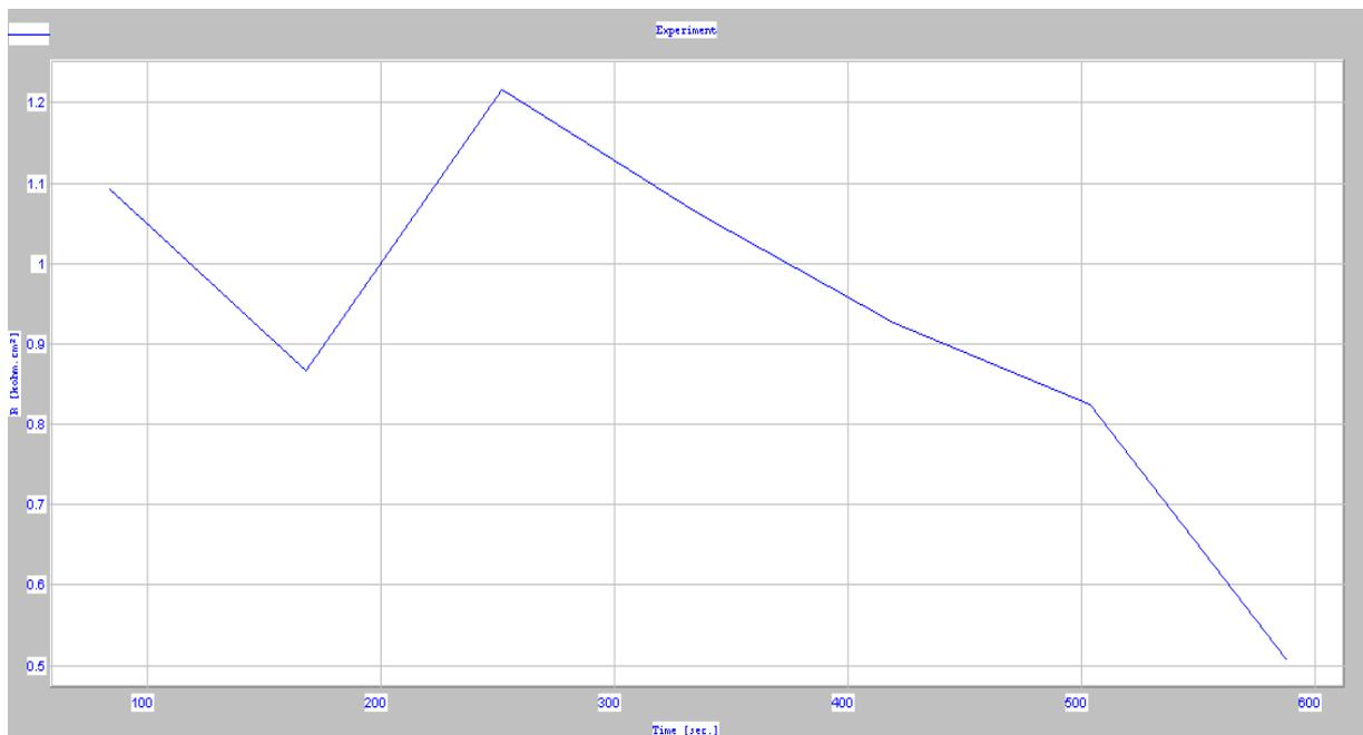
**Figure 5:** Polarization resistance function of time for the sample coated with Zn-Bi I
