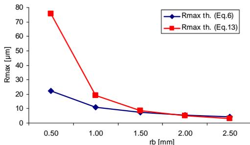
**Figure 5:** Theoretical results of roughness surface expressed with theoretical models at different deforming ball diameter
