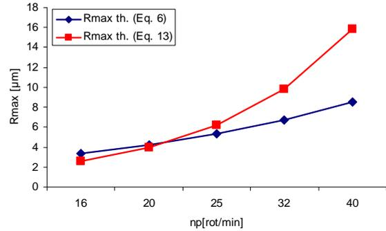
**Figure 6:** Theoretical results of roughness surface expressed with theoretical models at different part speed
