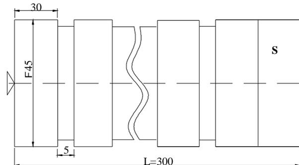
**Figure 4:** Dimensions and geometry of workpiece
