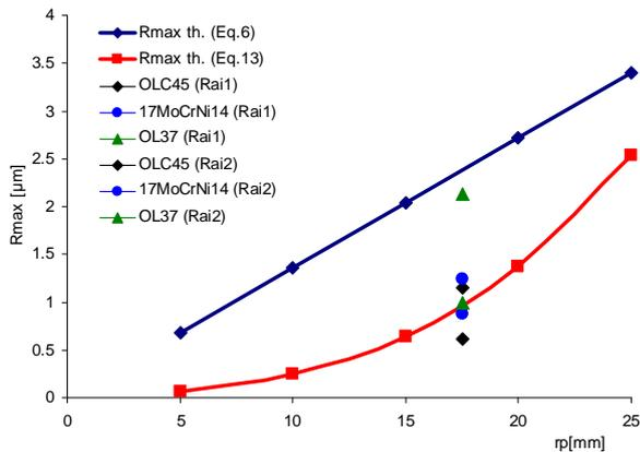
**Figure 8:** Theoretical results of roughness surface expressed with theoretical models at different part radius; experimental points, resulted in same working conditions, on different materials.
