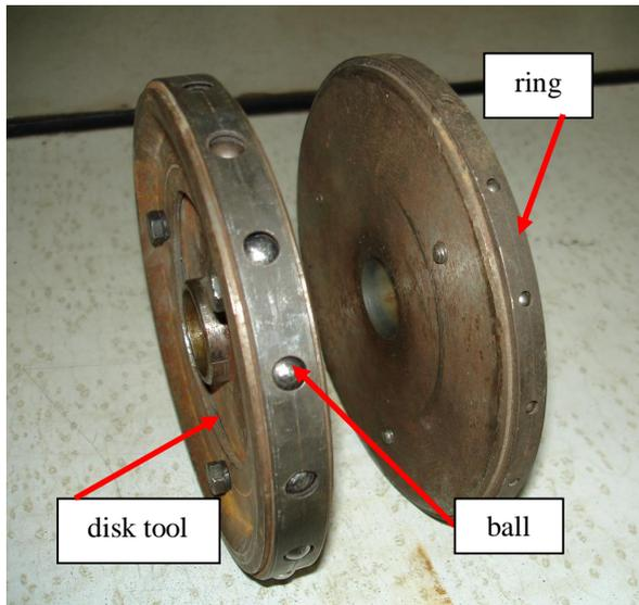
**Figure 3:** Disks with deforming balls (different diameters of balls).
