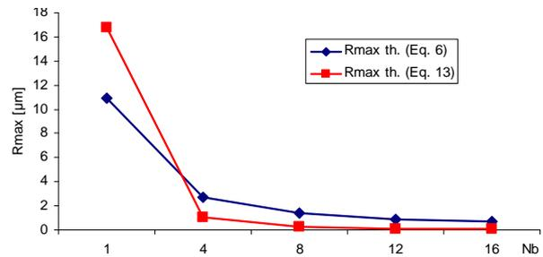
**Figure 7:** Theoretical results of roughness surface expressed with theoretical models at different number of balls on disk tool
