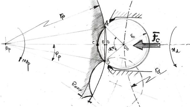
**Figure 1:** Schematic diagram of the smoothing process with centrifuged balls.
