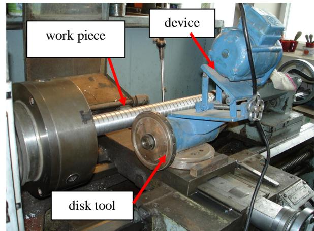
**Figure 2:** Device for smoothing by plastic deformation with centrifuged balls.
