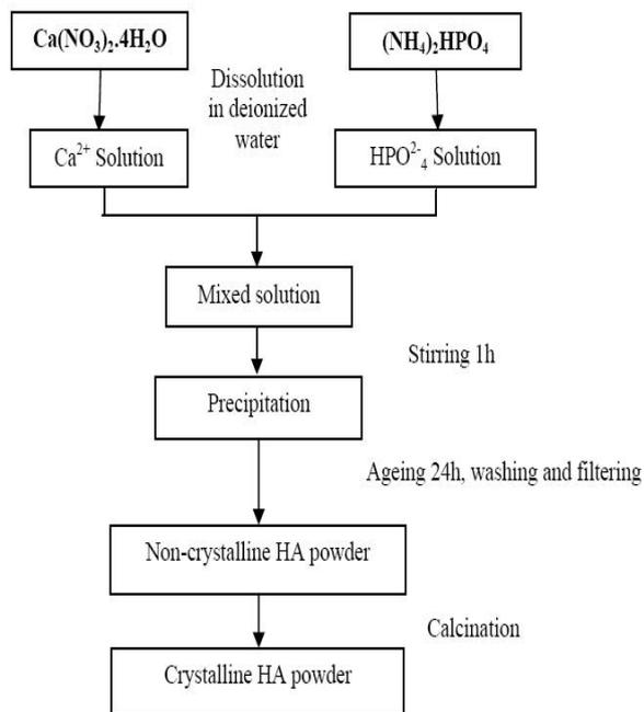
**Figure 1:** Modified chemical precipitation route for HA powder preparation. (Adapted from Sung) [3]
