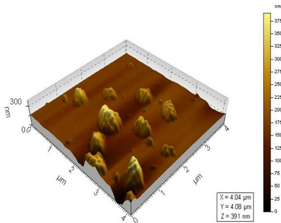
**Figure 12:** 3-D representation of the HA crystals obtained by wet precipitation
