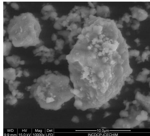
**Figure 10:** Electron microscopy SEM for Hap powder calcined at 1000°C, 10000 X
