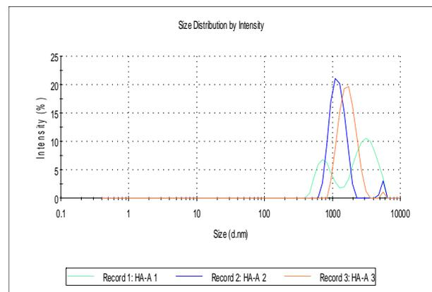
**Figure 2:** Size distribution of the three HAp samples after intensity
