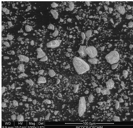
**Figure 9:** Electron microscopy SEM for Hap powder calcined at 1000°C, 1000 X
