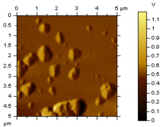
**Figure 11:** AFM image of the HA powder calcined at 1000°C
