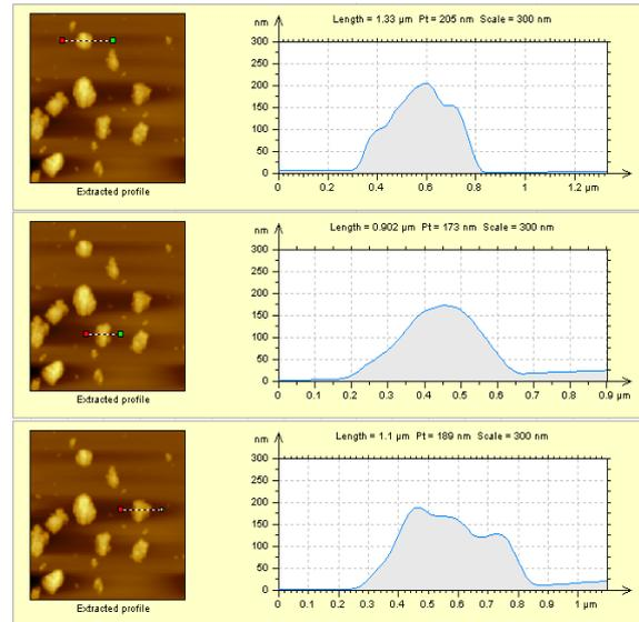
**Figure 13:** AFM analysis of hydroxyapatite powder
