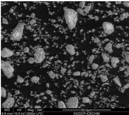
**Figure 8:** Electron microscopy SEM for Hap powder calcined at 1000°C, 2000 X.
