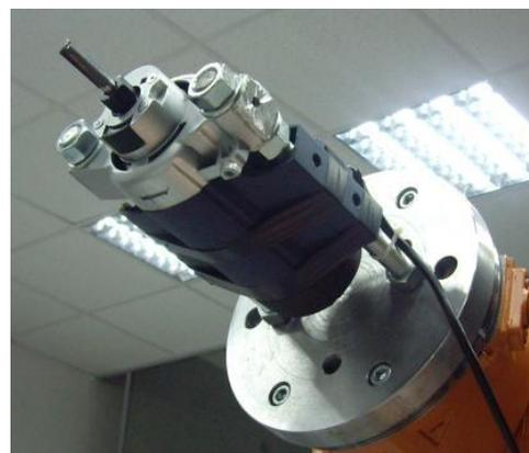
**Figure 6** – Milling device attachable to the robot Kuka KR125
