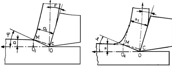
Figure 2.1: Cutting with a single shear plane
