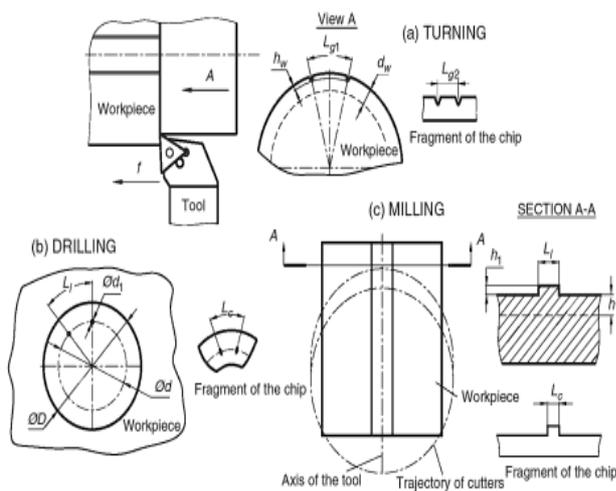
**Figure 2.2** Experimental methods to determine  $C_d$ : a. turning; b. drilling; c. milling.
