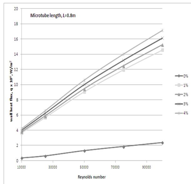
**Figure 4:** Particle volume fraction effect on the wall heat transfer flux:  $L=0.8m$  [4]
