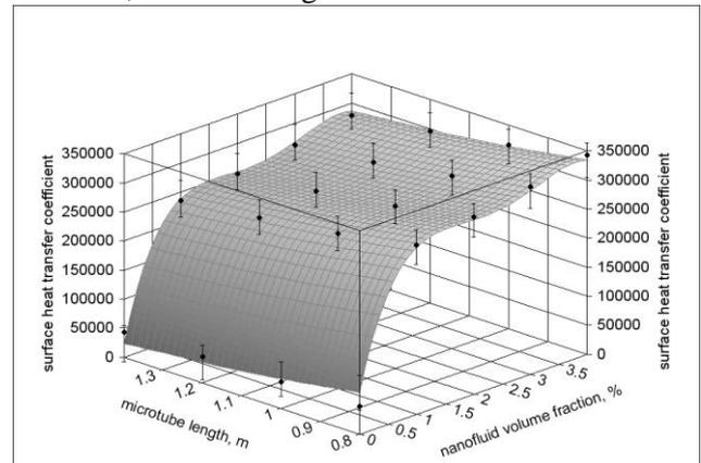
**Figure 7:** Heat transfer coefficient evaluation based on microtube length and nanofluid volume fraction for Re=10<sup>5</sup> [4]
