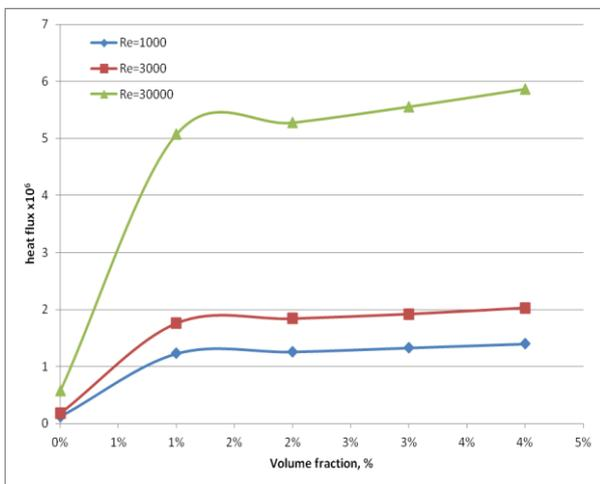
**Figure 8:** The influence of the particle volume fraction  $\phi$  on the wall heat transfer flux
