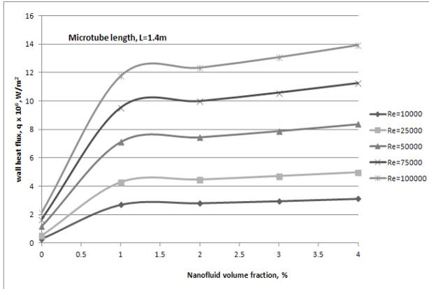
**Figure 5:** Reynolds number effect on the wall heat transfer flux: L=1.4m [4]
