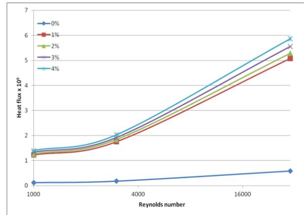
**Figure 9:** The influence of the Reynolds number on the wall heat transfer flux
