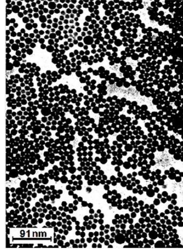
**Figure 1:** TEM image of the alumina nanoparticles after dispersion [5]
