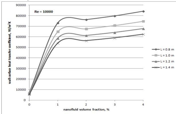
**Figure 6:** Effect of the tube length on the heat transfer [4]
