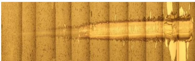
Figure 8: Photo of the sign from Scratch test for  $ncAlTiN/\alpha Si_3N_4$  coating over 100Cr6 steel
