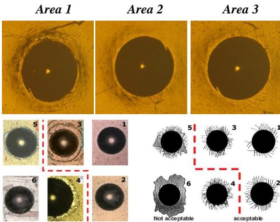
Figure 7: Experimental imprints obtained for coating TiN compared with the adhesion evaluation criteria
