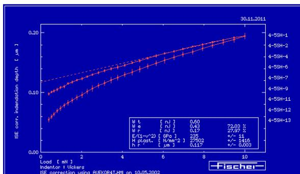
Figure 13: Load-unloading diagram of the process for hardness measuring of  $TiN$  coating
