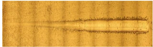
Figure 9: Photo of the sign from Scratch test for  $ncAlCrN/\alpha Si_3N_4$  coating over 100Cr6 steel
