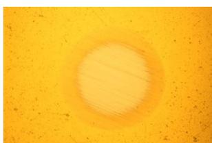
**Figure 3:** Photo of imprint to determine the thickness of coating  $TiN$  over 100Cr6 steel
