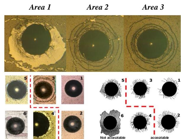
**Figure 5:** Experimental imprints obtained for coating  $ncAlTiN/\alpha Si_3N_4$ , compared with the adhesion evaluation criteria
