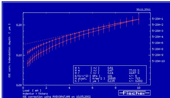
Figure 12: Load-unloading diagram of the process for hardness measuring of  $ncAlCrN/\alpha Si_3N_4$  coating
