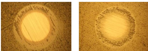
**Figure 2:** Photos of imprints to determine the thickness of coatings  $ncAlTiN/\alpha Si_3N_4$  and  $ncAlCrN/\alpha Si_3N_4$  over 100Cr6 steel
