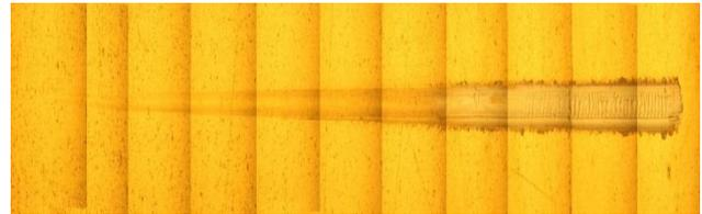
Figure 10: Photo of the sign from Scratch test for TiN coating over 100Cr6 steel
