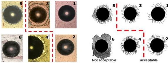
Figure 6: Experimental imprints obtained for coating  $ncAlCrN/\alpha Si_3N_4$ , compared with the adhesion evaluation criteria
