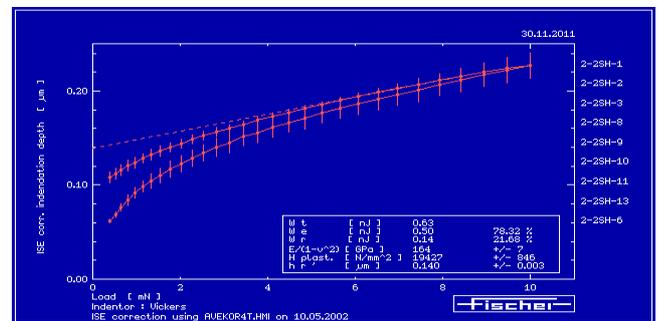
Figure 11: Load-unloading diagram of the process for hardness measuring of  $ncAlTiN/\alpha Si_3N_4$  coating
