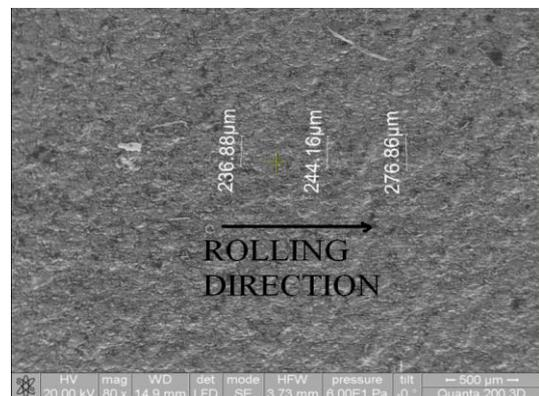
**Figure 2:** The appearance and the size of impression left on the sample with lubricant
