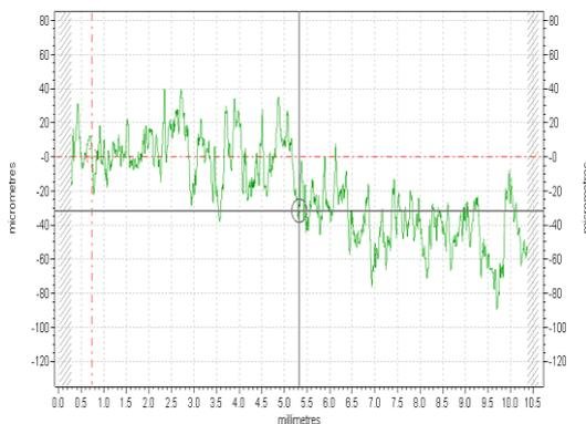
**Figure 13:** The shape of the wear trace under lubricant friction condition
