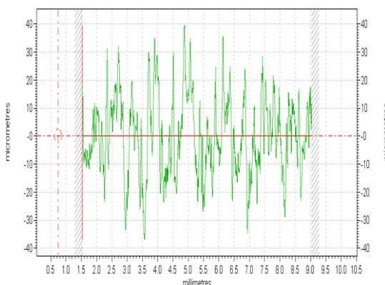
**Figure 14:** The roughness values of the sample in lubricant friction condition
