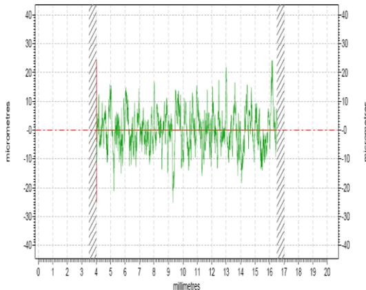
**Figure 8:** Roughness values in condition of friction disk with the lubricant
