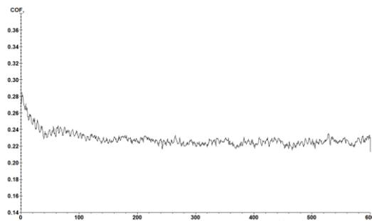
**Figure 6:** The variation of the friction coefficient from the pin-disk test in lubricant friction conditions
