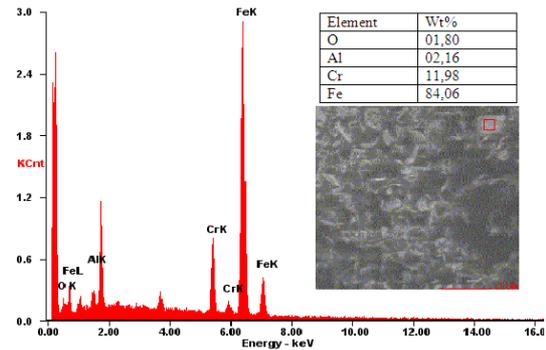
**Figure 5:** SEM and EDAX analysis of the residual powder after the friction test
