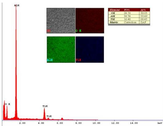
**Figure 4:** Map distribution of the elements and EDS analyses of the wear
