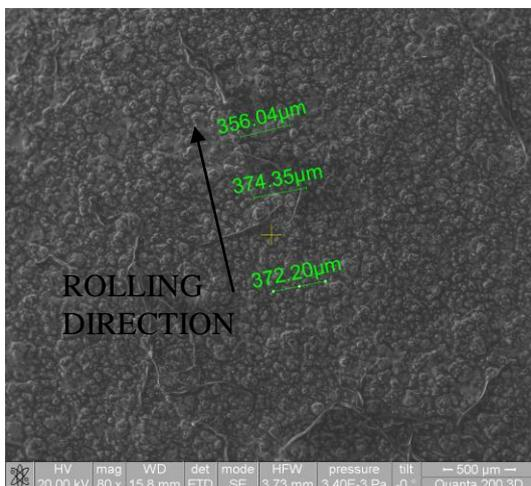
**Figure 9:** The appearance and the size of impression left on the sample with lubricant
