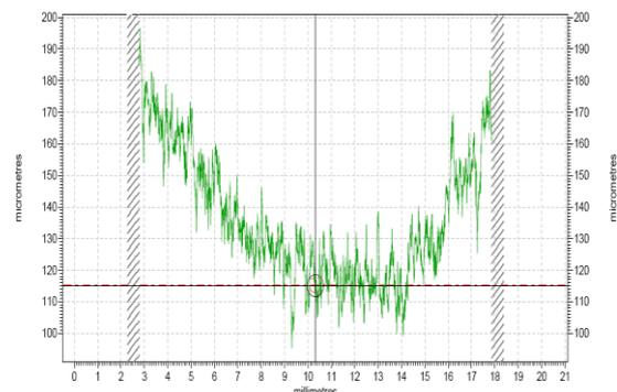
**Figure 7:** The form of the channel due to wear in conditions of lubricant friction
