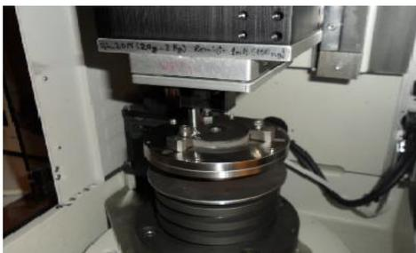
**Figure 1:** The way how the sampled is mounted on the CETR UMT-2 tribometre
