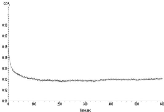
**Figure 12:** The variation of the friction coefficient from the pin-disk test in lubricant friction conditions
