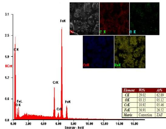
**Figure 11:** The distribution map of the chemical elements and the EDS
