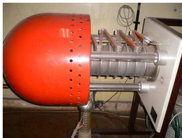
**Figure 2:** Neutron generator used for fast (14 MeV) NAA in metallurgical industry (ISW Galati)
