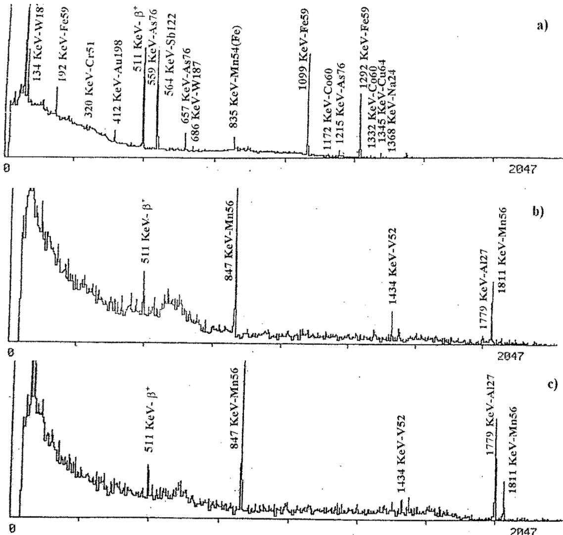
**Figure 1:** Gamma rays NAA spectra of a steel sample obtained at IFIN-HH for long (a) and short (b) irradiation and spectrum of an iron ore for short irradiation (c).
