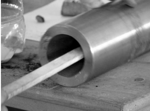
Figure 15: Metallic shell for casting alloy.
