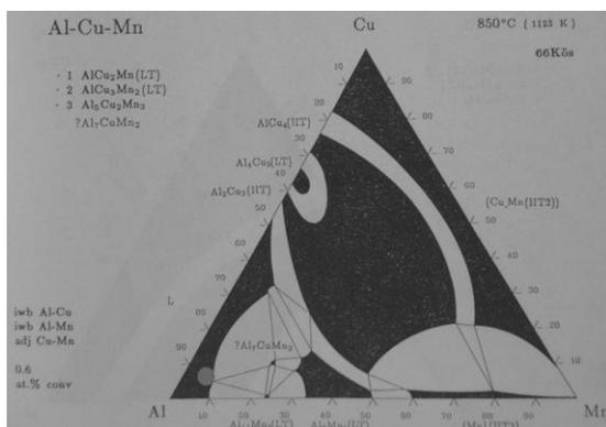
Figure 9: Cu-Al-Mn ternary diagram at 850°C temperature [6].
