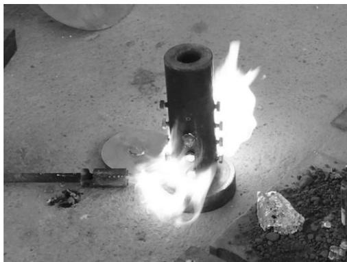
Figure 16: Shell preheating before casting alloy.
