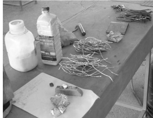
Figure 12: Dosage of alloying elements, in accordance with calculating the load elements.
