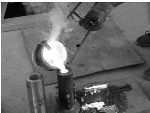
Figure 17: Casting the alloy.
