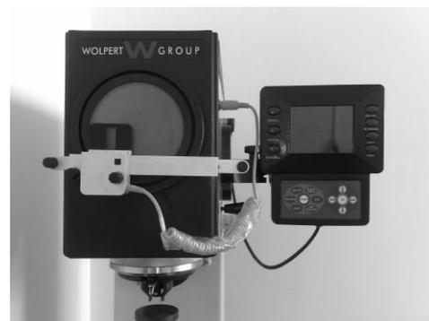
Figure 19: Wilson Wolpert universal hardness tester model 751N.
