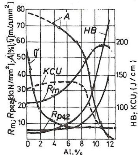
Figure 2: Influence of aluminium on mechanical characteristics of aluminium bronzes.
