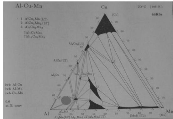
Figure 10: Cu-Al-Mn ternary diagram at 20°C temperature [6].
