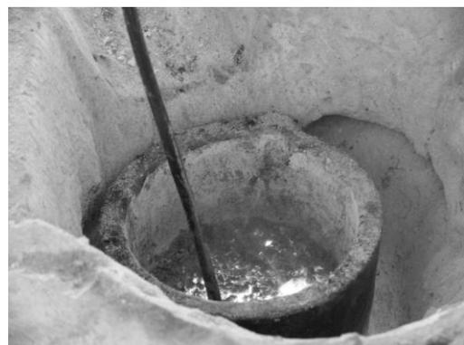
Figure 14: Homogenization of alloy.
