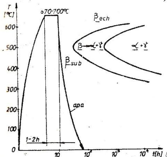
Figure 11: TTT diagram chart quenching and Cu-Al eutectoid alloy with 11.8% Al.
