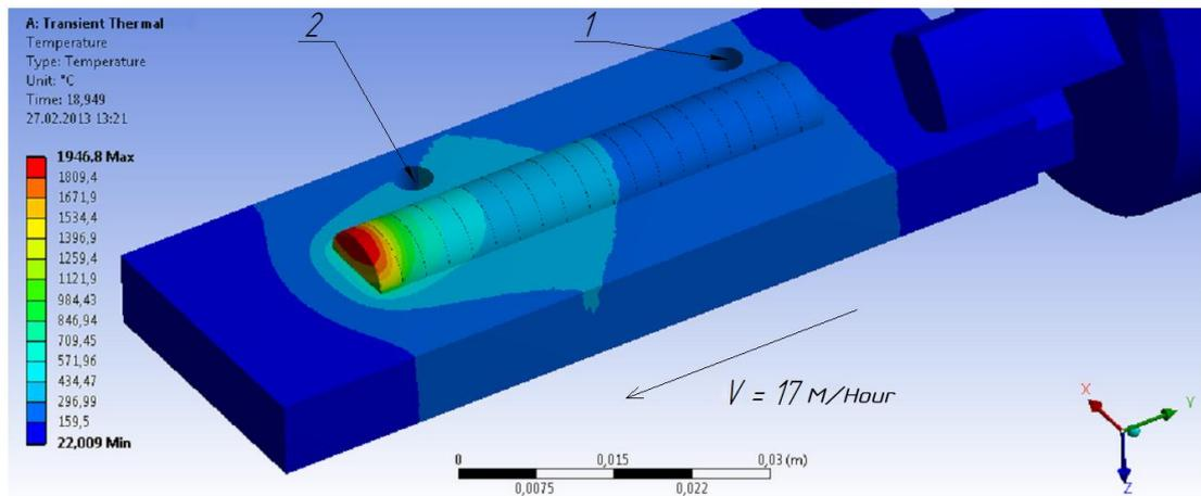
Figure 1: Plate Temperature Field during Fusion
