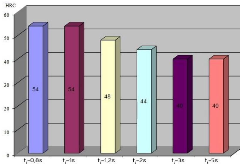
**Figure 6:** Hardness of Fused Samples
