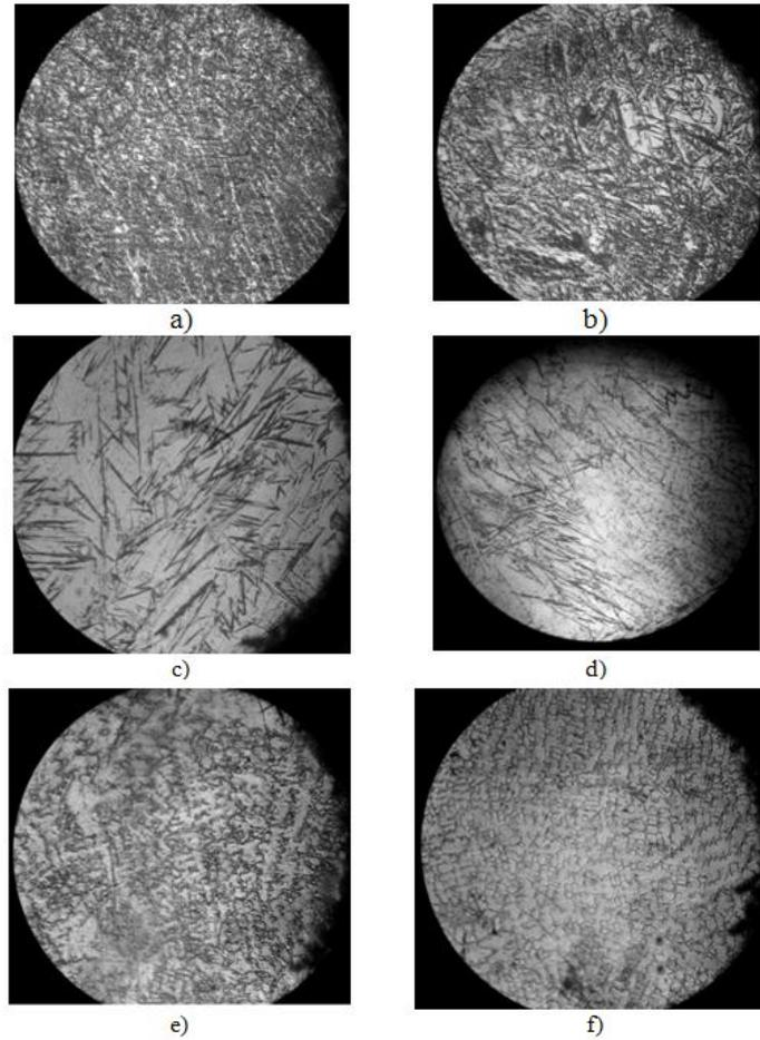
**Figure 5:** High-Carbon Fused Coating Microstructure ( $\times 150$ ):
