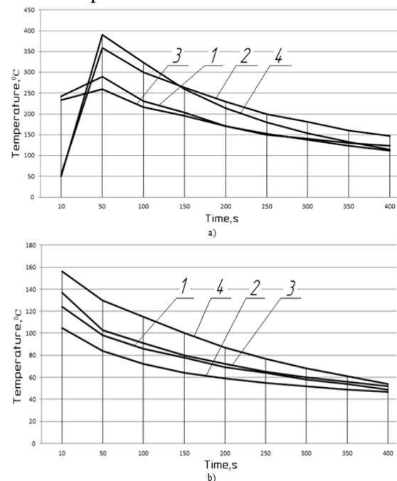
Figure 2: Temperature Variations in Sample Preset Points in the Course of Fusing and Cooling: a)  $t_{amp} = 5$  s; b)  $t_{amp} = 1$  s.
