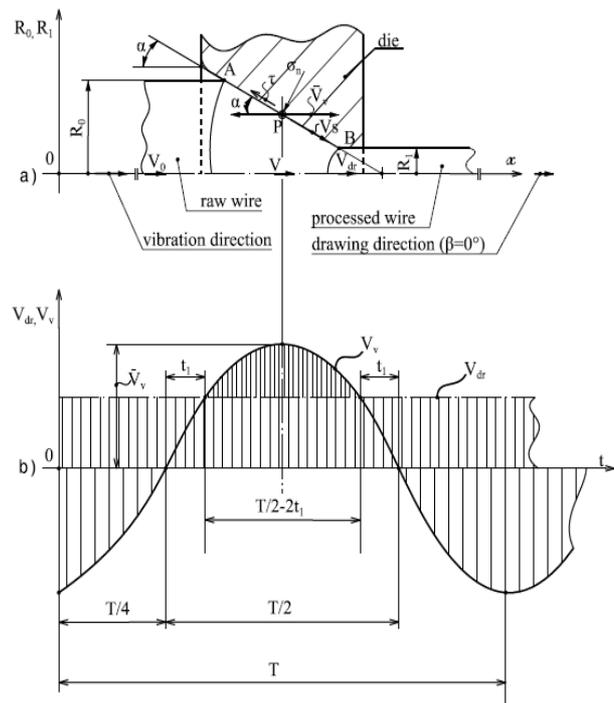
**Figure 2** Procedure of plastic deformation by drawing, during the ultrasound drawing-UVD of the metallic wires with cylindrical symmetry:
