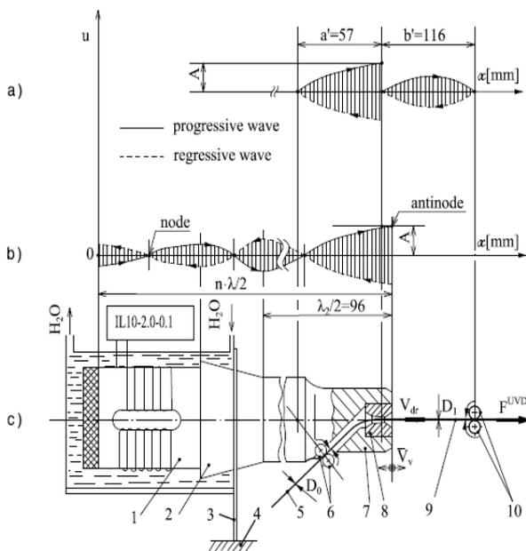
**Figure 5:** Scheme of the oscillator system used for the experimental research:
