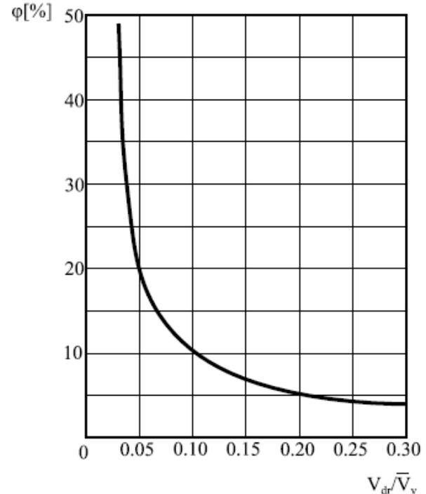
**Figure 4:** Variation of the coefficient ( $\varphi$ ) in function of the relative rate of drawing ( $v_{dr}/\bar{v}_v$ ), for a given ultrasound drawing process-UVD:  $D_0=3.50\text{mm}$ ;  $D_1=3.00\text{mm}$ ;  $\alpha=8^\circ$ ;  $\delta_i=19\%$ ;  $f=22000\text{Hz}$ ;  $\lambda_i=1.18$ ;  $v_{dr}=0.06\text{m/s}$ ;  $A=25\mu\text{m}$ ;  $v_v=3.45\text{m/s}$ .
