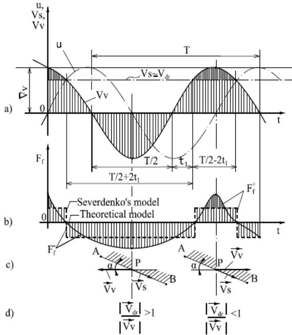
**Figure 3:** Kinematics of the plastic deformation by drawing-U VD technology:
