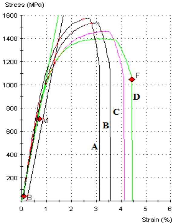
**Figure 6:** Cumulative diagram of the drawing stress, samples A, B, C, and D.
