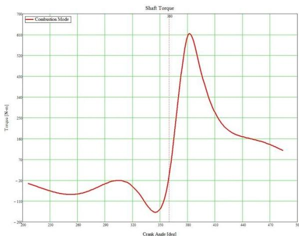
Figure1: The instantaneous torque for combustion mode.
