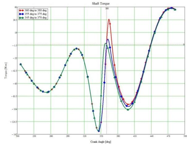
Figure2: The evolution of torque for different angles to open or close the exhaust valve.
