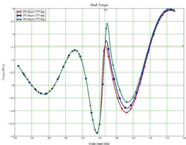
Figure4: Torque evolution for constant closing angle of exhaust valve.
