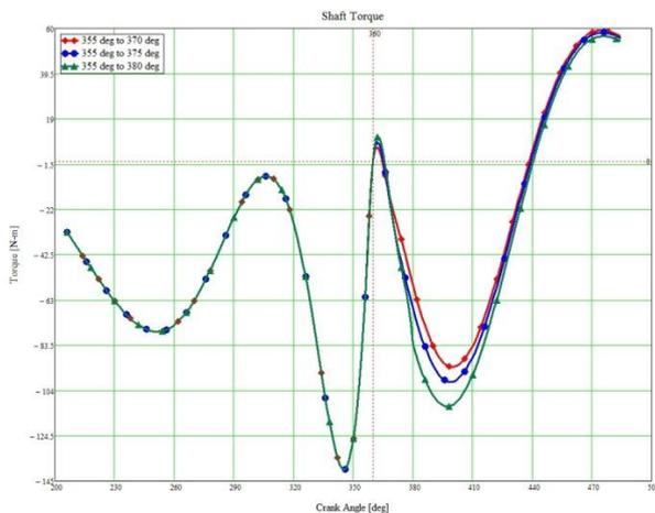
Figure3: Torque evolution for constant opening angle of exhaust valve.
