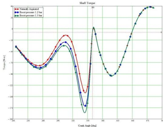
**Figure 5:** The evolution of torque with the pressure supply.
