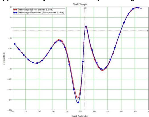
**Figure 6:** The evolution of torque with the air fresh cooling
