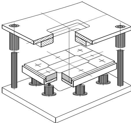
**Figure 2:** Die with segmented blank-holder, [12] rectangular parts application
