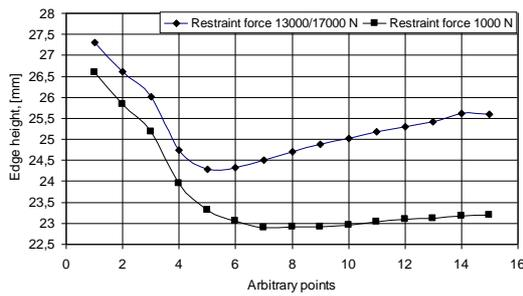
Figure 8: Edge height in the smaller lateral zone
