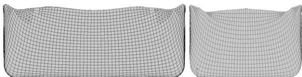
Figures 11: Edge form of the part for a compose binder force of 13000/17000 N
