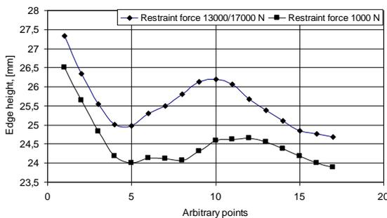
Figure 9: Edge height in the longer lateral zone
