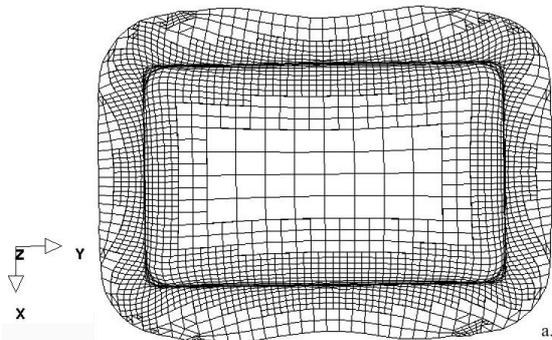
**Figure 6:** The intermediate shape of the blank in FEM simulation, constant force
