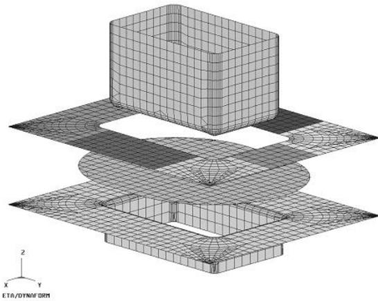
**Figure 5:** The tooling used in FEM simulation
