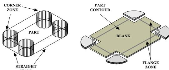
**Figure 3:** The geometry of a rectangular part and corresponding blank, [2]
