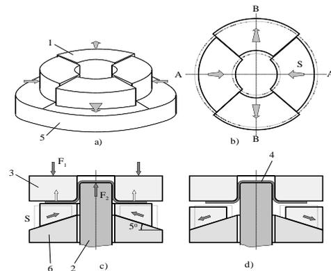
**Figure 1:** Die with segmented blank-holder, cylindrical parts application [13]
