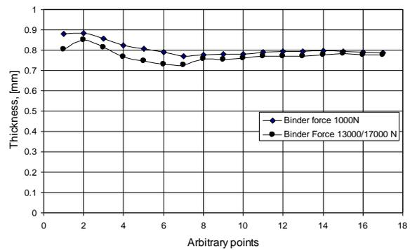
Figure 12: Thickness variation in the smaller lateral zone
