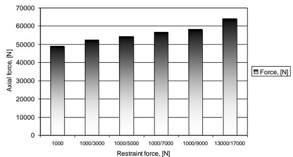
Figure 14: Axial force variation in rectangular panel deep drawing
