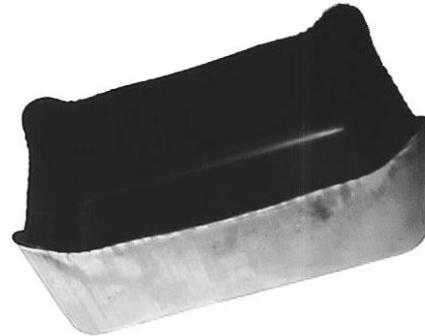
**Figure 18:** The shape of the rectangular part for a binder force of 1000 N
