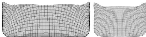
Figure 10: Edge form of the part for a constant binder force of 1000 N
