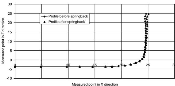
**Figure 16:** Panel springback for a compose binder force of 13000/17000 N
