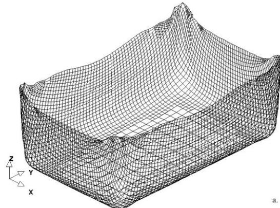
**Figure 7:** The final shape of the blank, for a binder force of 1000 N
