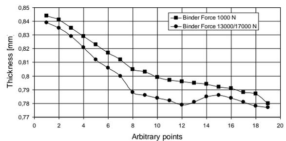
Figure 13: Thickness variation in the longer lateral zone
