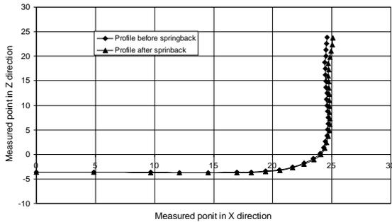
**Figure 15:** Panel springback for a binder force of 1000 N
