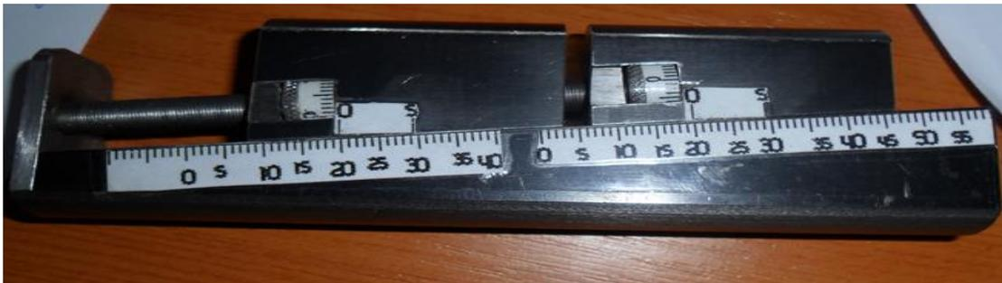
**Figure 3:** Adjustable “pass” - “do not pass” caliber with the reading system type “linear graduated scale - circular graduated vernier”
