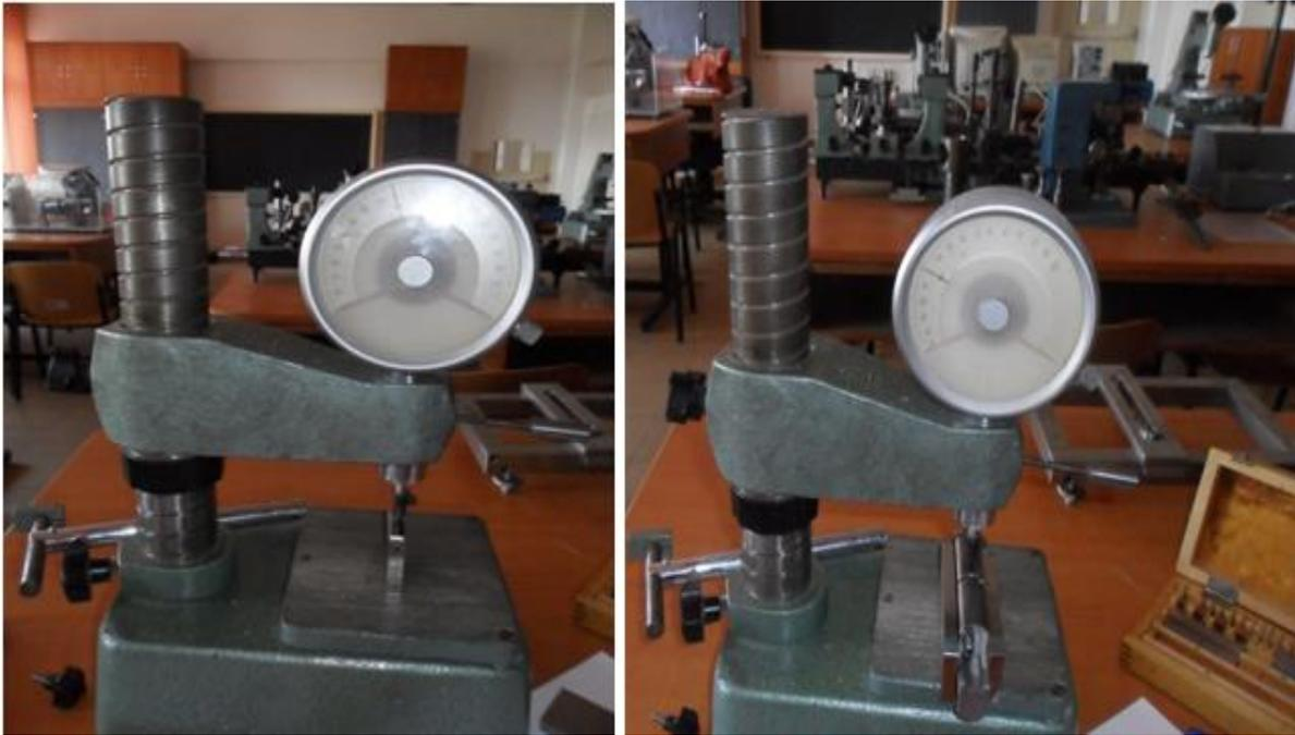
**Figure 4:** Adjustment to "zero" for the adjustable "pass" - "do not pass" calibers
