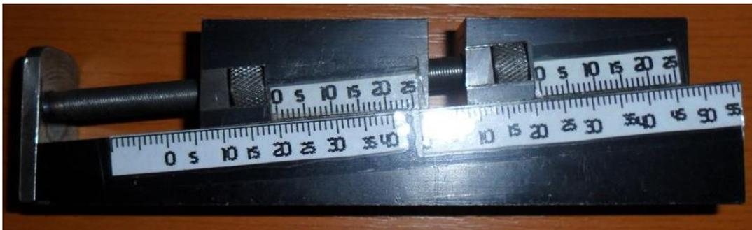
**Figure 5:** Adjustable "pass" - "do not pass" caliber with the reading system type "linear graduated scale - linear graduated vernier"
