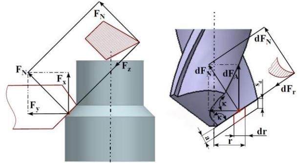
**Figure 3:** Analogy turning-drilling. The components of the cutting forces [Ștețiu, 1994]
