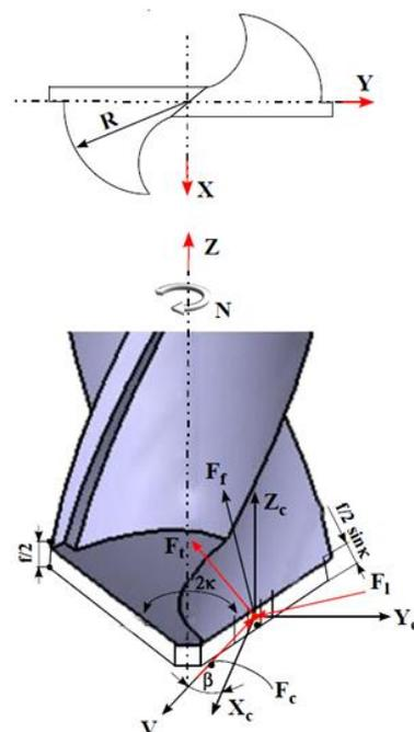
**Figure 1:** Correlation between forces in orthogonal cutting and drilling [Yang, 2002]
