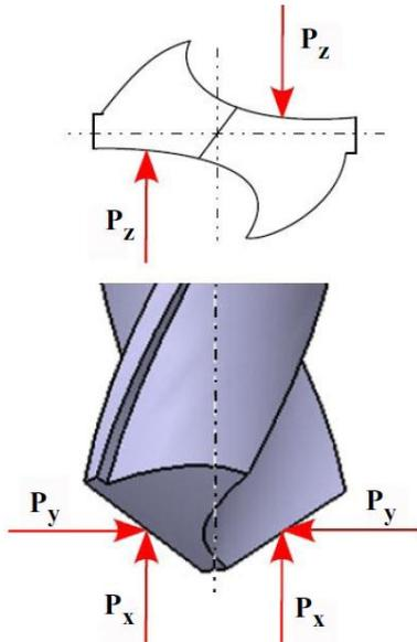
**Figure 2:** Components of the cutting forces [Minciu, 1999]
