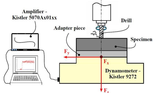
**Figure 4:** Block diagram of the experimental installation [Baroiu,2013]
