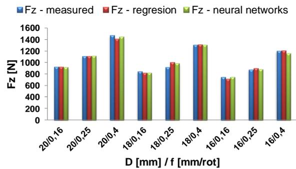
Figure 8:  $F_z$  force at the machining A570
