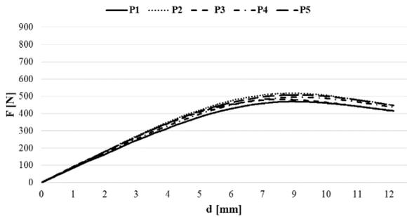
Figure 3: Force-displacement curve for epoxy Resin.
