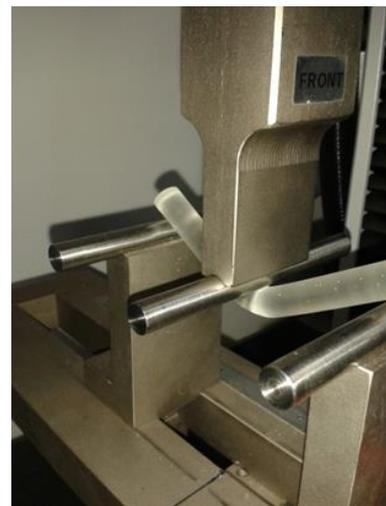
**Figure 2:** The bending specimen sample.
