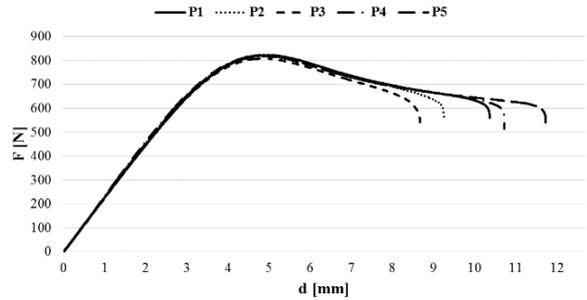
Figure 6: Force-displacement curve for PU2
