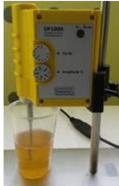
**Figure 1:** Ultrasonic Processor UP100H during epoxy treatment.
