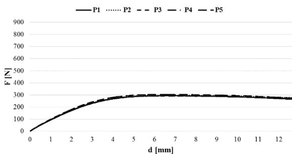
Figure 5: Force-displacement curve for PU1
