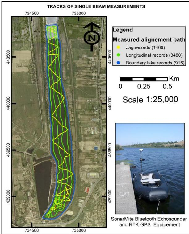
Figure 4. Jag and longitudinal method of depth measurements
