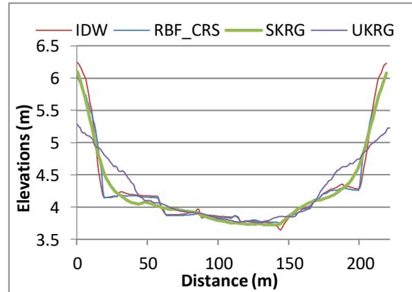
Figure 8. Cross section profile 1-2, represented in figure 8, from different interpolation method
