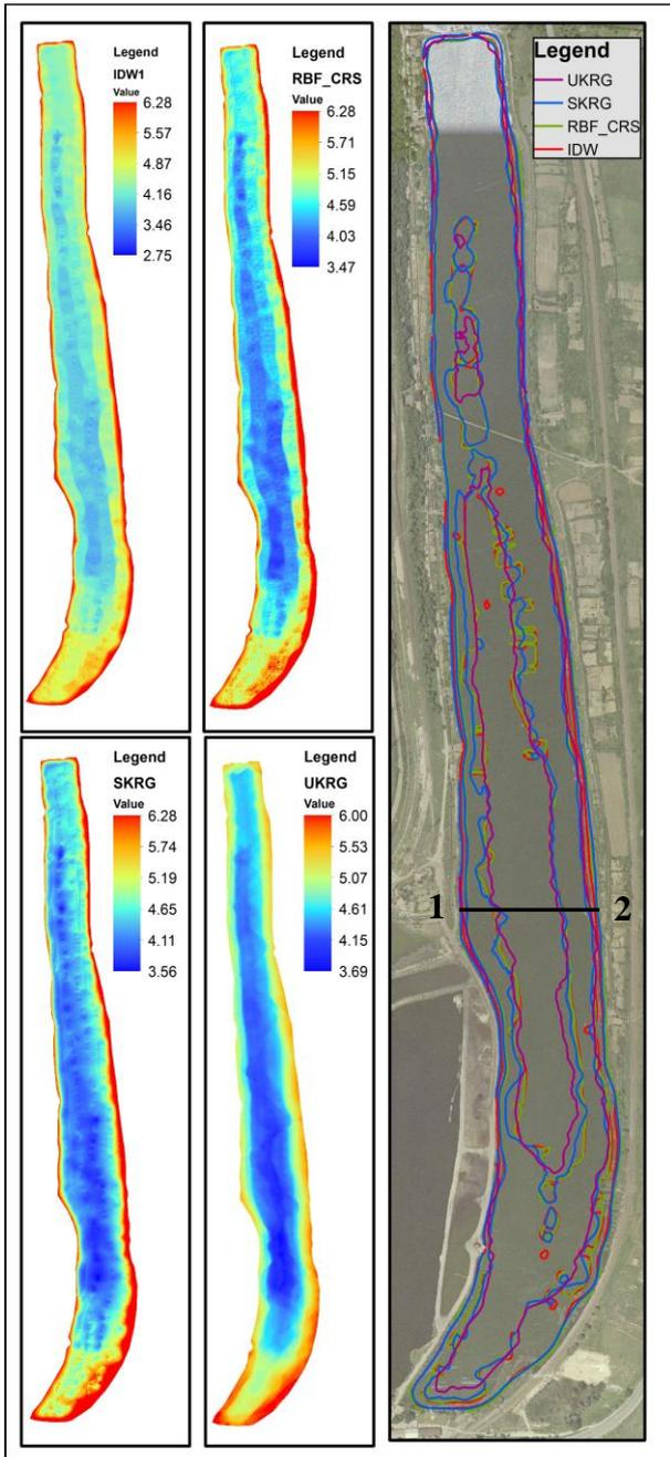
Figure 7. The obtained bathymetric models and 1 meter depth contours
