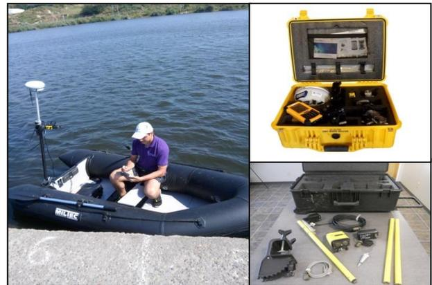
Figure 3. Used instruments and mounting method on an inflatable boat
