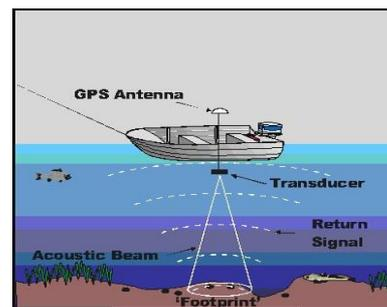
Figure 1. Depth measurement with a singlebeam echosounder (<http://www.ozcoasts.gov.au>)
