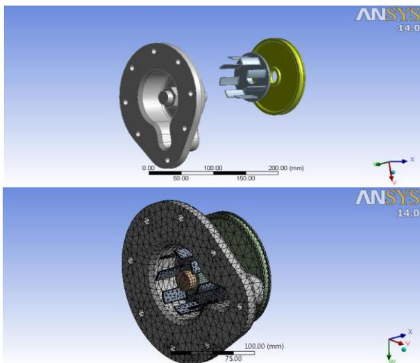
**Figure 13:** Pump's part for assembly and mesh using ANSYS-Mechanical library-2017
