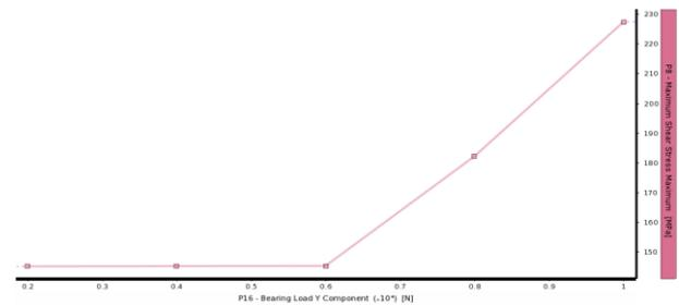
**Figure 11:** Diagram max shear stress related to bearing load applying on Lever in various cases with AL material- using ANSYS-Post
