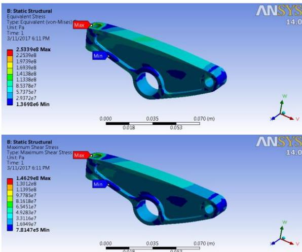
**Figure 9:** Equivalent stress and Shear stress distribution (respectively) on Lever in case study No.2 with steel- using ANSYS-Structural software
