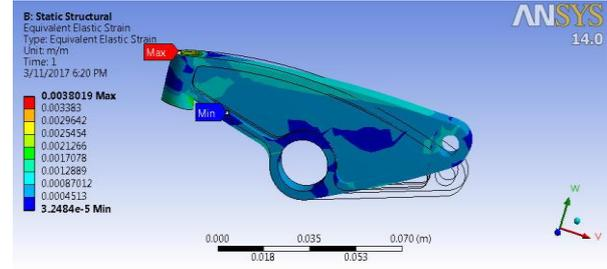
**Figure 10:** Equiv. strain and total deformation distribution (respectively) on lever in case No.2 with steel mat.-using ANSYS-Structural software
