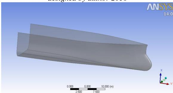
**Figure 3:** Delta bow model for ship using ANSYS-DM software designed by author 2016
