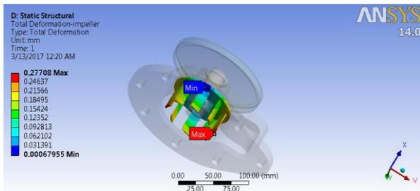
**Figure 16:** Total deformation for impeller under 1000 N load- using ANSYS-Mechanical software
