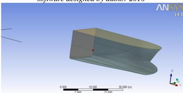
**Figure 4:** Oval bow model for ship using ANSYS-DM software designed by author 2016
