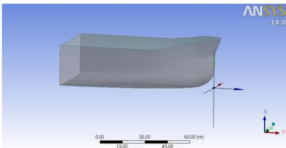
**Figure 2:** Flat bow for ship using ANSYS-DM software designed by author 2016
