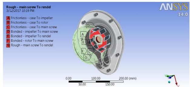
**Figure 14:** Pump assembly contacts definition- using ANSYS-Mechanical
