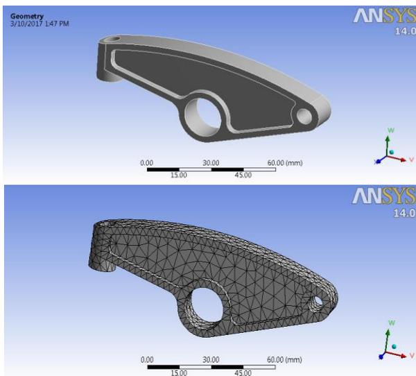
**Figure 7:** CAD model for Lever part and the mesh of elements using ANSYS-DM software-2017
