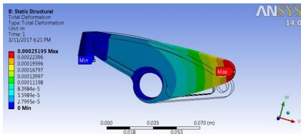
We can isolate one parameter and analyze the changes in its value in all cases like what we showed in Fig. 11, where the relation between bearing load and maximum shear stress appears. Based on material properties the designer has to define the critical points which maybe will carry critical values for shear, normal or equivalent stress, these points
