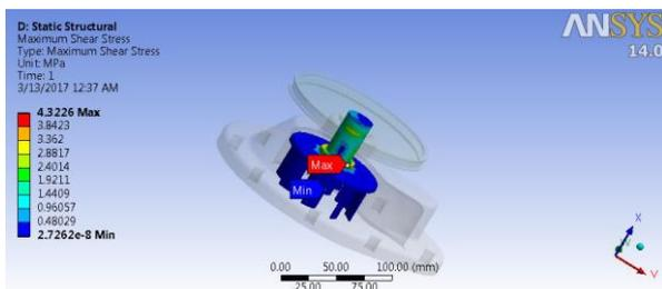
**Figure 17:** Shear stress distribution under 1000 N loads- using ANSYS-Mechanical software
