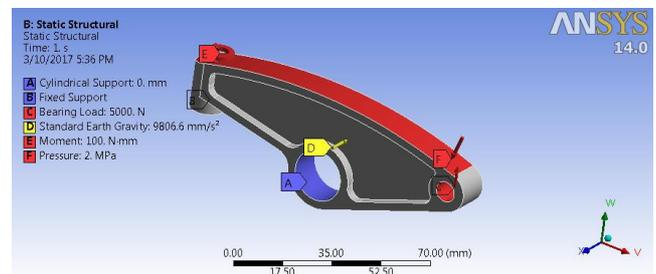
**Figure 8:** Boundary conditions and forces applied on lever model using ANSYS-Structural Analysis
