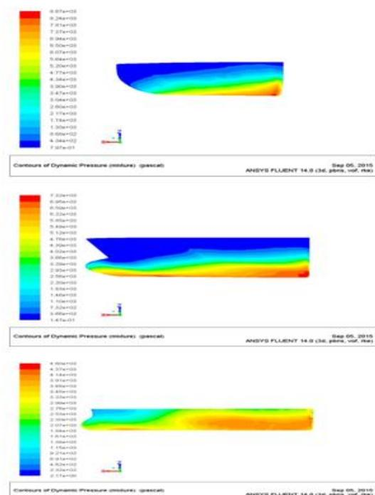
**Figure 5:** Hydrodynamic pressure distribution on hull for Flat-Oval and Delta bows using ANSYS-FLUENT software, designed by author 2016
