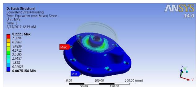
**Figure 15:** Equivalent stress distribution on pump housing under 1000 N load- using ANSYS-Mechanical software
