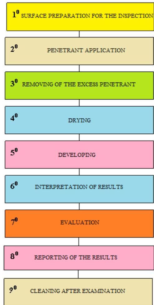
Figure 2: Steps of liquid penetrant inspection
