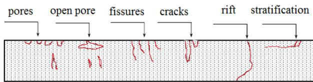
Figure 1: Types of defects
