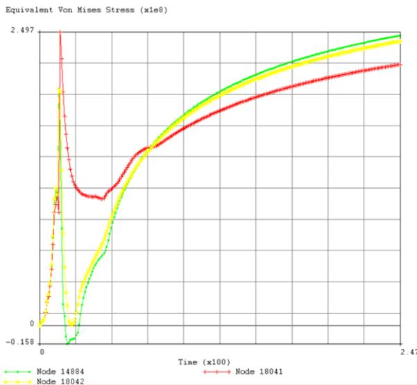
**Figure 6:** The variation curves of the Von Mises stress in quasi-stationary thermal field, in time, for three nodes situated in the welding axis.
