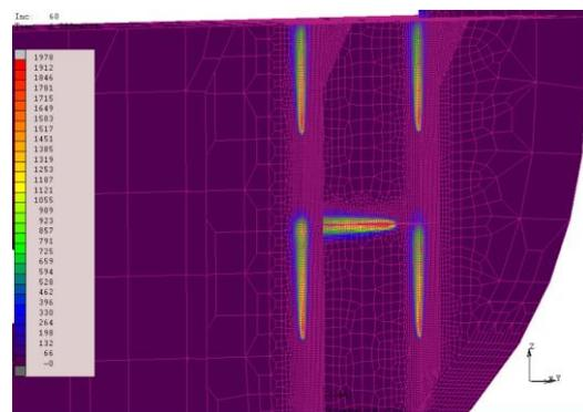
**Figure 2:** Location of the five heat sources after the process starting ( $t=60s$ )
