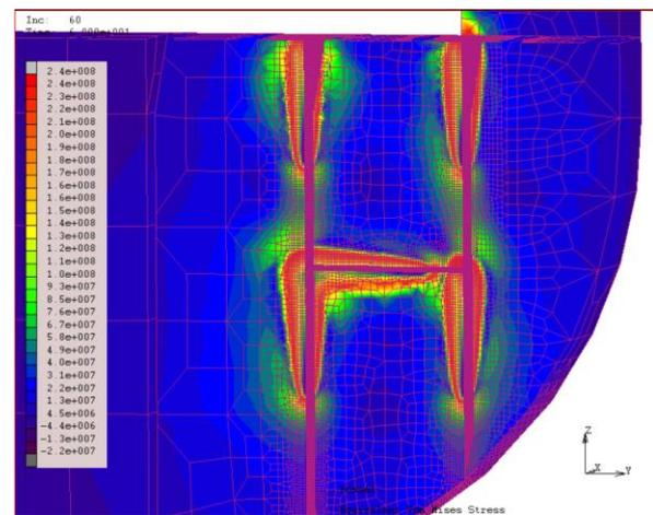
Figure 5: The Von Mises stresses distribution in plate after 60s
