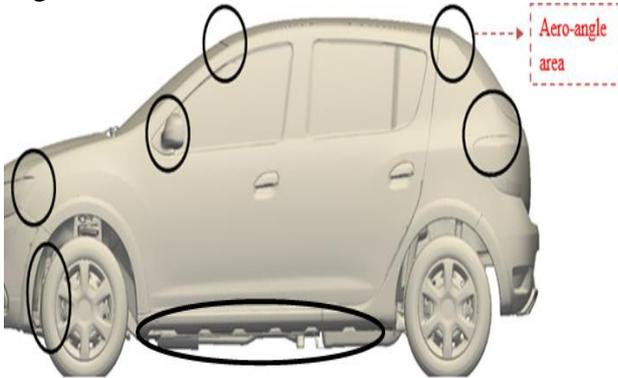
**Figure 6.** High sensitive areas of aerodynamic behavior of the vehicle
