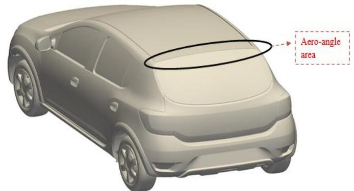
**Figure 7:** The aero-angle area for the Initial Model of the vehicle
