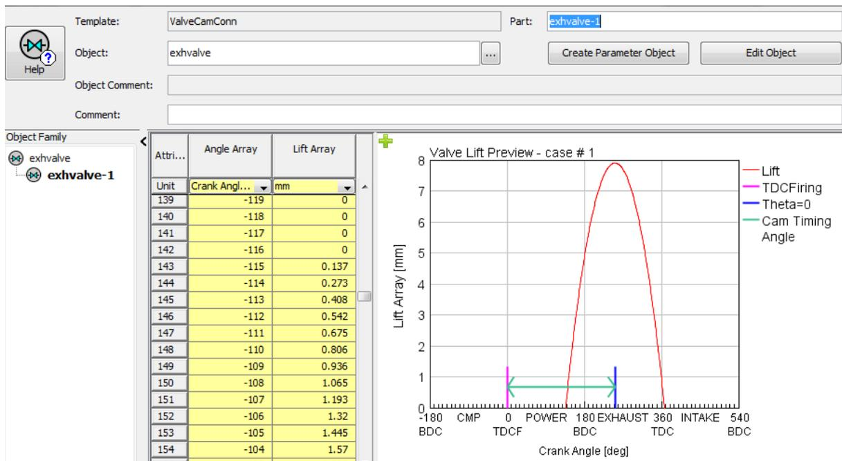
Figure 4: Exhaust valve modeling
