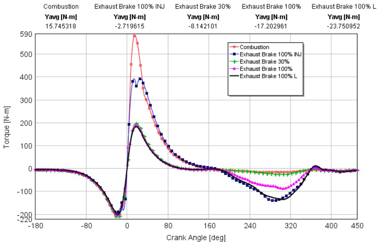
**Figure 10:** Evolution of engine torque
