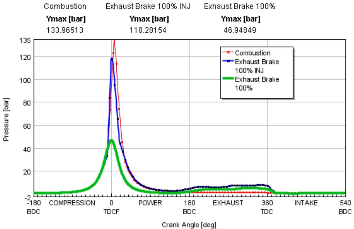
Figure 8: In cylinder pressure evolution
