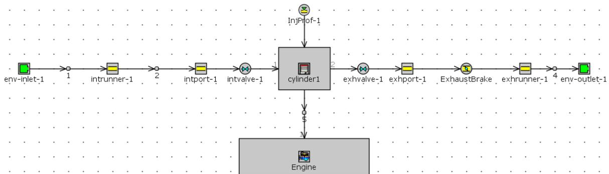
**Figure 2:** Block diagram of the single cylinder engine
