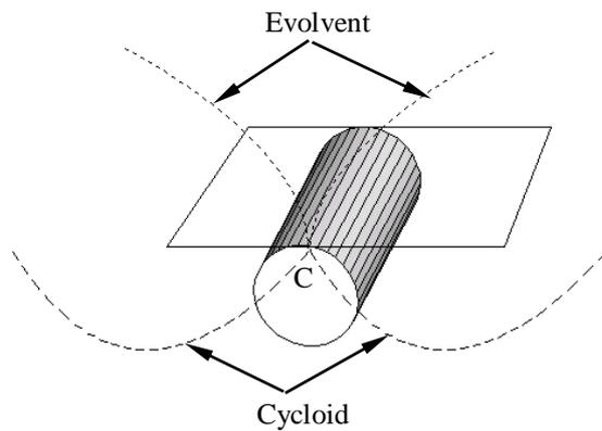
**Figure 4** Irreversibility of cylinder-plane contact
