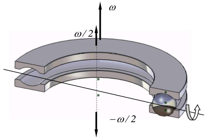
**Figure 6** Axial section through a thrust ball bearing
