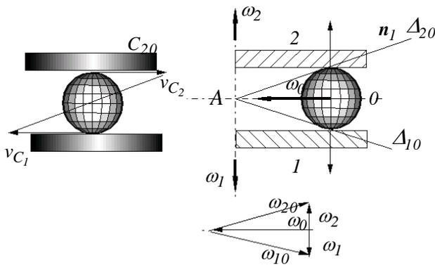
**Figure 7.** Distribution of velocities in a thrust ball bearing
