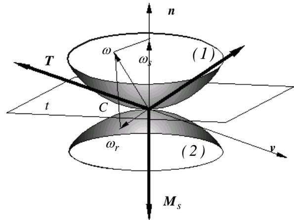
**Figure 5.** The relative motions and the torsor of friction in a point contact
